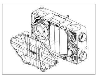
5. Unscrew the heat exchanger retaining clamps (4 x) one turn and slide them out.
