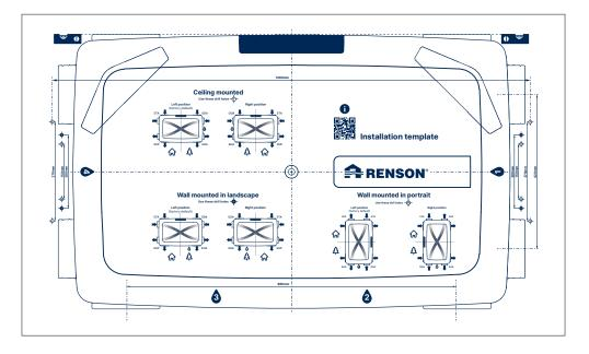
**3.** By measuring directly on the bracket with the dimensions indicated here. Renson recommends using method 1 or 2, unless one is used to working without these tools. In this case you can use the bracket & drawing with dimensions in this manual.
