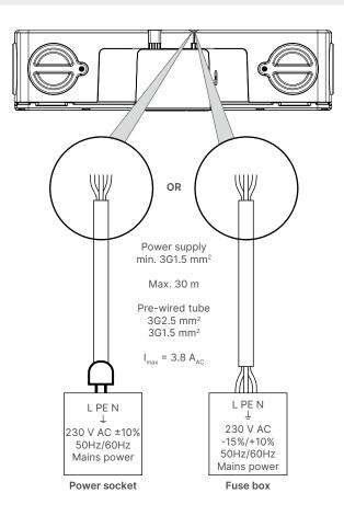
The installation and electrical connection of the various components may only be carried out by authorised personnel in accordance with the applicable safety measures.
