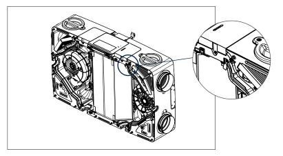
6. Remove the heat exchanger.
