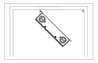
**9.** Ensure the unit is securely attached by tightening the supplied 3xM6 bolts in combination with the knurled spring washer and flat washer at the indicated locations (see figure).
