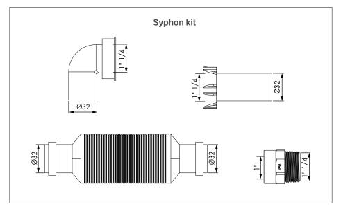
To ensure you have a correct water drainage point without odour nuisance, it is strongly recommended to use the Renson siphon kit for Flux Go Flat. Follow the instructions on the supplied sheet carefully to ensure proper functioning of the unit.
