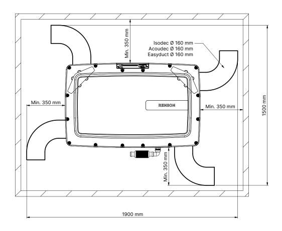
Some examples of set-ups in practice can be seen below, taking into account the above minimum distances and the Renson recommendation to always provide 1 m Acoudec  $\emptyset$  160 mm on the supply and extraction sides. This will give you a whisper quiet installation.
