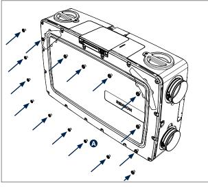
Loosen all 16 UPVC screws (A) before removing the cover.
