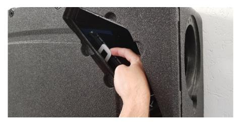
Step 3 • Pull the connection box out a little so you have access to the sensor.
