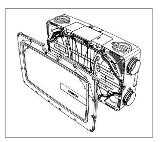
3. Unscrew the tabs (B) of the condensation collection tray (C) one turn and turn the tabs a quarter turn.
